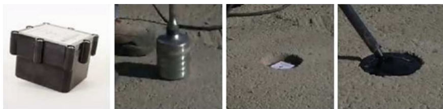
Fig. 4 Example of a vibration sensor [33]
