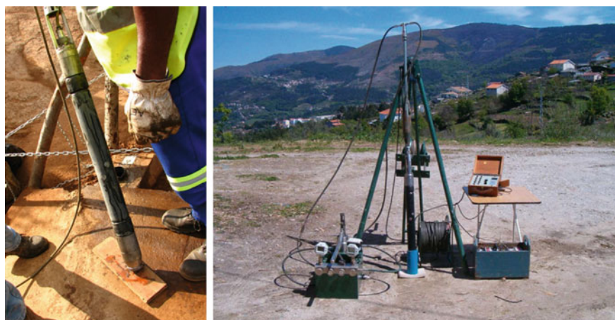
Fig. 18 BHD dilatometer probe ( left ) and full equipment ( right )
