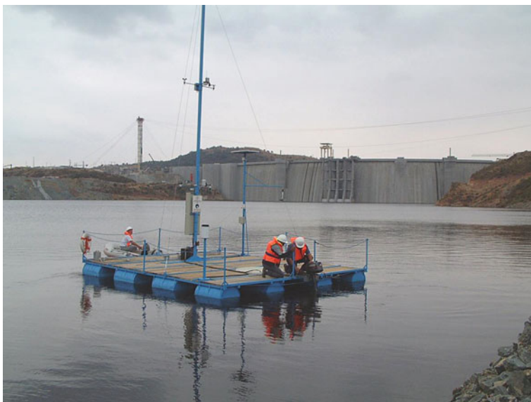
Fig. 2 Assembling and setting up a floating meteorological station, with underwater sensors for temperature and water quality implemented in the man-made lake of Alqueva in southern Portugal
