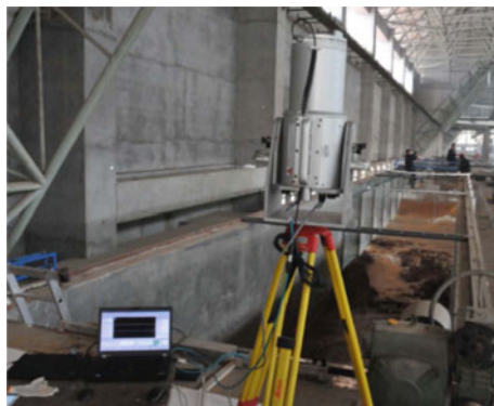
Fig. 17. 3D scanner used in dam-breaching tests
