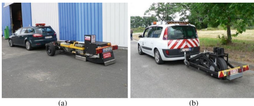
Fig. 12 Trailers for rolling resistance measurements, based on the angle measurement principle: a TU Gdansk trailer; b BRRC trailer. Photos by Anneleen Bergiers
