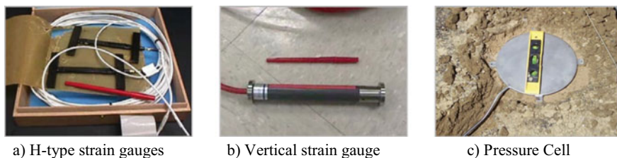
Fig. 2 Sensors for pavement instrumentation: strain, deformation, and pressure measurements
