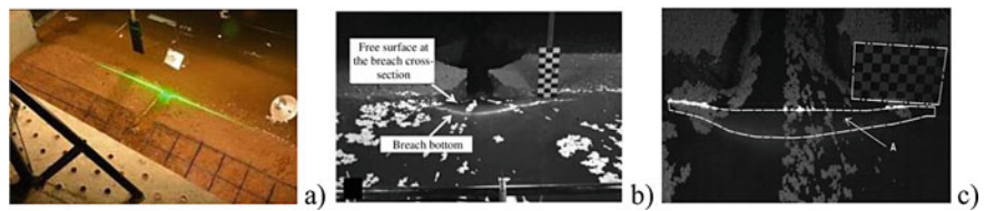
Fig. 12 a Laser sheet projected in the dam, right upstream the crest; b image acquired with the upstream high-speed camera (Photonfocus—Fig. 10) illustrating the laser traces projected at the dam body and at the free-surface; c breach area determined by approach A
