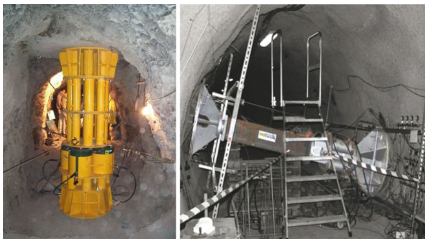
Fig. 19 Plate loading tests in an adit (left) [45], and in a tunnel (right) [46]
