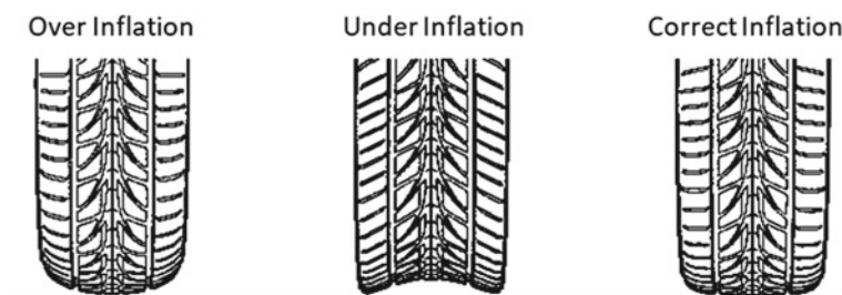
Fig. 11 Treadprint area for different tyre pressure. Adapted from https://www.bridgestone.com.sg/en/tyre-clinic/tyre-talk/tyre-tread-wear-causes
